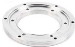
Titanium nitride hardening protects the contact surfaces for the suction-side ring plates, and considerably improves resistance against abrasive wear caused by contact with the piston rings.
