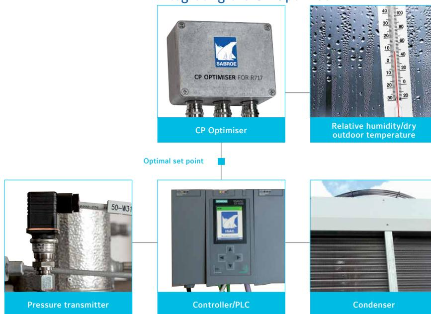
Temperature and relative humidity sensors are not included with the Sabroe CP Optimiser, but are available as optional equipment. Controller (PLC) not included.
