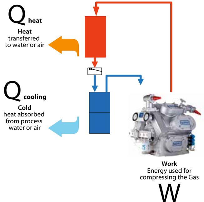
Figure 3: In a typical dairy you cool the milk when it arrives to the dairy and when it is processed. During pasteurisation of milk it is heated to about 80°C using steam produced in a boiler that supplies a hot water loop. This hot water can be heated by a heat pump rather than a boiler.
