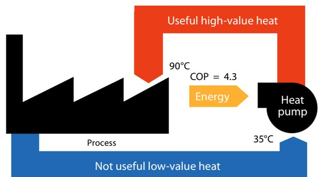
Figure 4: Reusing the low-value heat you can produce hot water with high efficiency compared to a state-of-the-art boiler.
