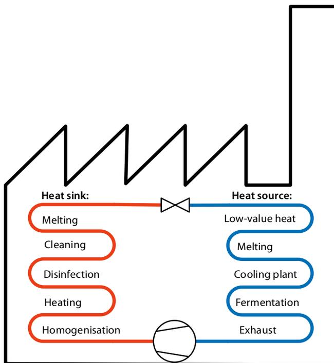
Figure 7: In industrial process heat pumps, the cold side is used for recovering heat or cooling a product. As shown in figure 6, the heating can be gained at a low level and sent to the right, where the temperature level is higher. If you cannot use the cooling or heating capacity internally then consider the possibility of selling the capacity to others in the neighbourhood.
