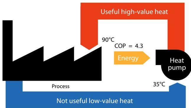
Figure 2: In industrial processes you produce low-value heat that is normally ejected to the ambient. With a heat pump this “waste heat” is transformed in to useful high-value heat, which can be used elsewhere in the process or sold for other uses.
