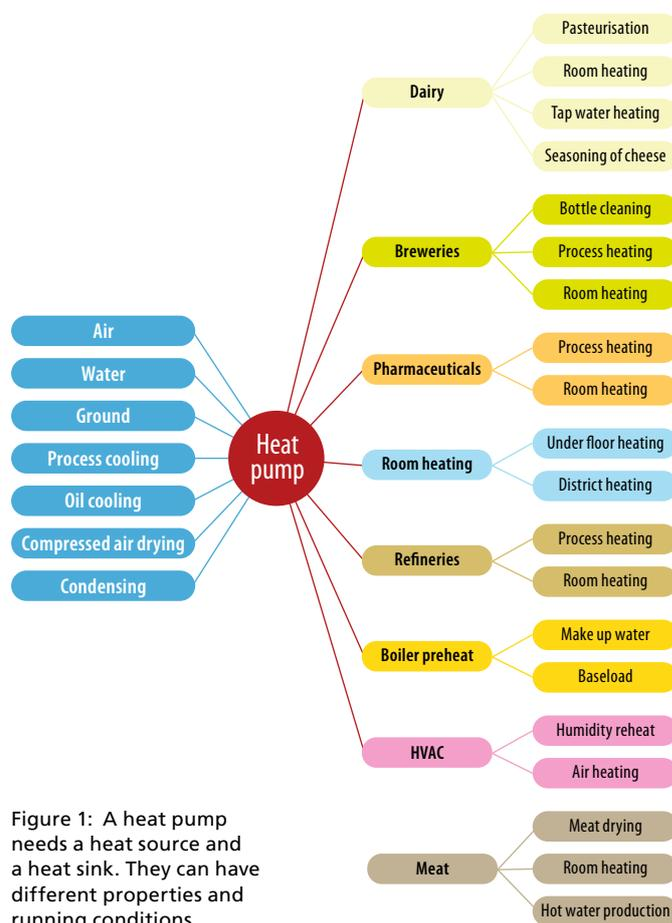
Figure 1: A heat pump needs a heat source and a heat sink. They can have different properties and running conditions.
