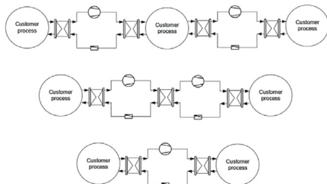
Figure 6: Three system layouts for heat pumps. The imagination sets the limits of how to connect and use heat pumps. Lower temperatures are to the left and the high temperatures to the right of the systems.
