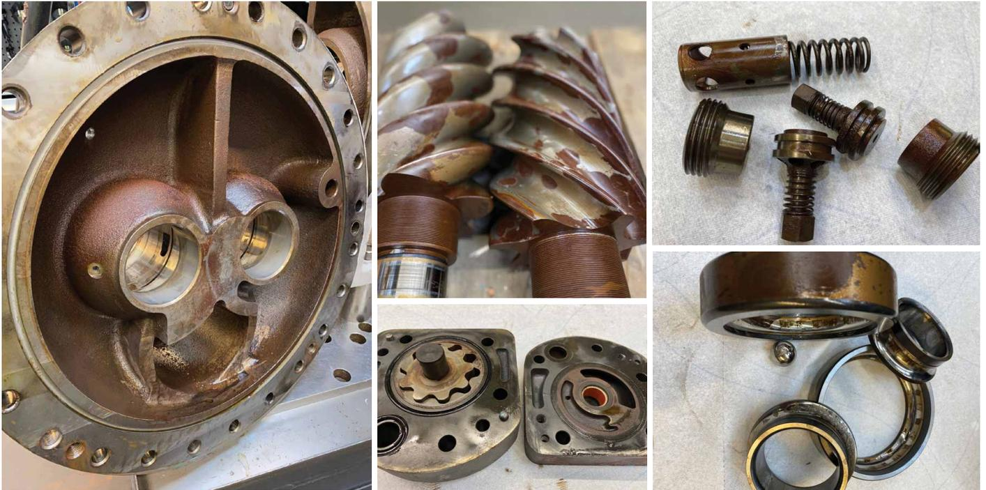
At Reman work shop, 25% of the compressor overhauls shows water contamination.
